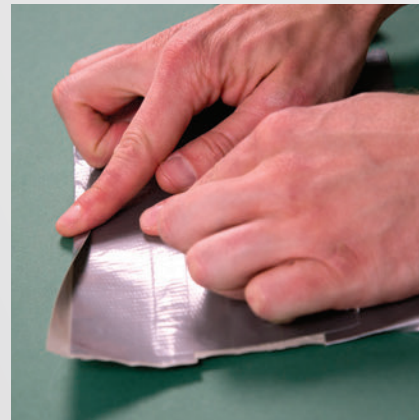
STEP 4: Fold and adhere the 1" duct-tape strips to the 9" ends of the sheet. This will make a smooth, clean finished edge.
